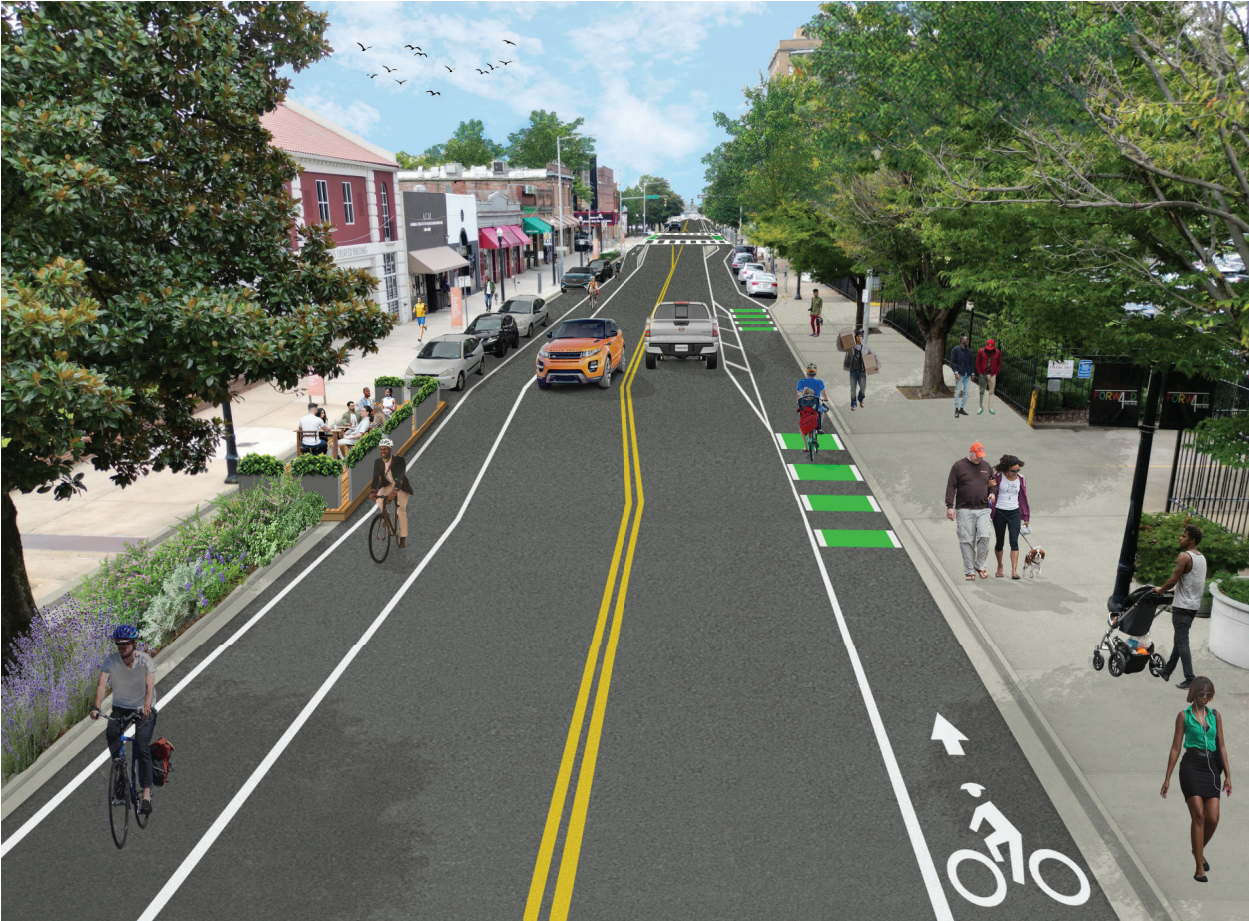
Figure 3. Photosimulation of corridor improvements. 4th Ave N will be converted to a two-way street, providing for bike and pedestrian facilities and on-street parking where possible, especially in the Business District.
